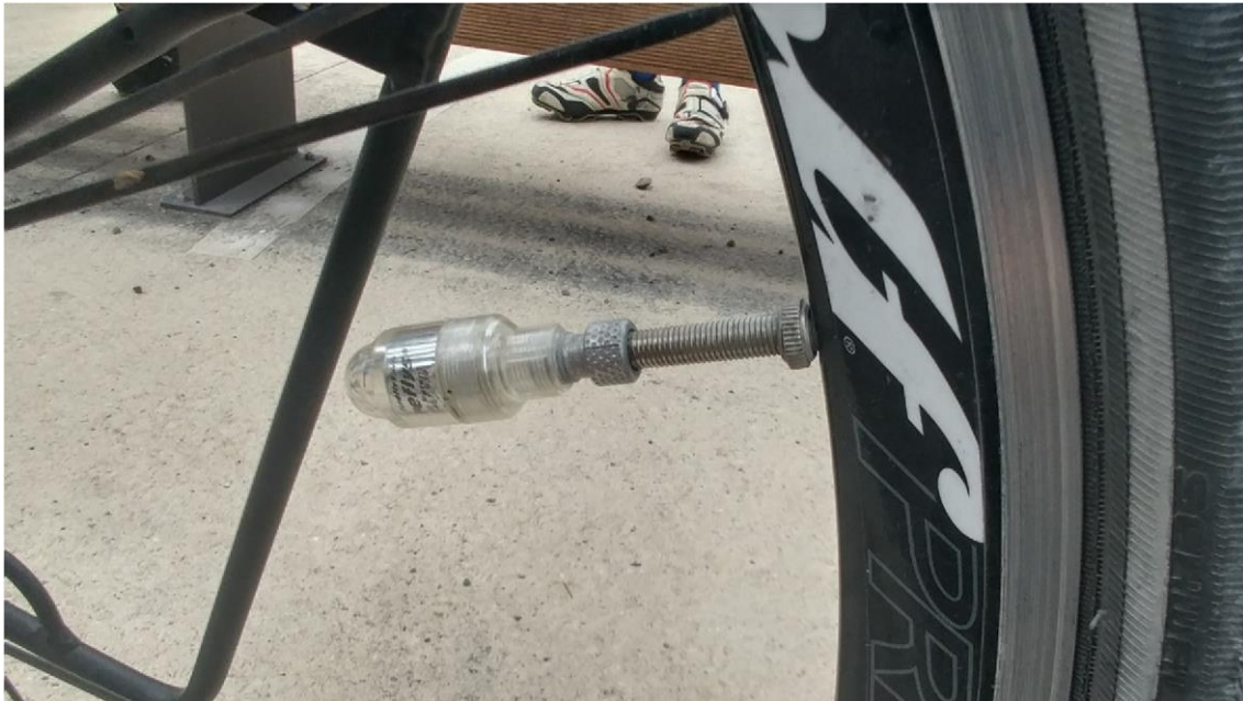
Presta Pressure Monitoring Valve Linked By Bluetooth To Smartphone App
