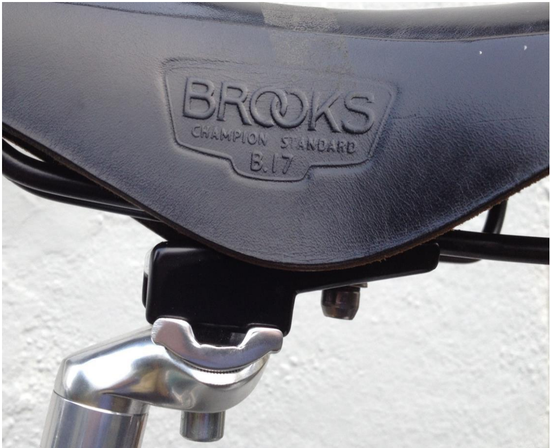
The VK Saddle Adjuster Allowing Greater Saddle Set Back
