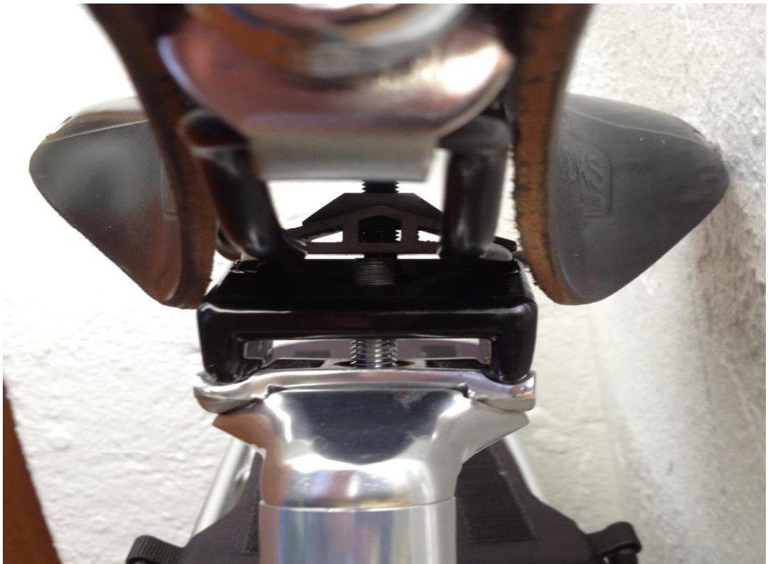
The VK Saddle Adjuster Allowing Greater Saddle Set Back
